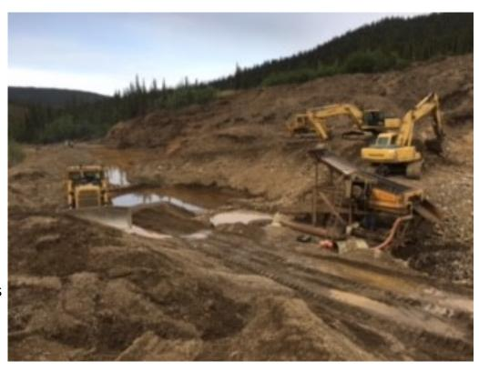
it. All the way in the back left is the water pump at the far end of a settling pond. They pump the water up to the plant and load the gravel with the excavator sitting right above it. The plant washes the gravel down and the gold stays in the sluice box which is underneath the shaker. The rest of the gravel goes into the pond, and they dig it out
